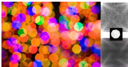
Figure 1. It is evident that the image's frequencies are multiplied by the bokeh kernel's frequencies because in spatial domain the kernel's characteristic is present in every pixel of the image.
